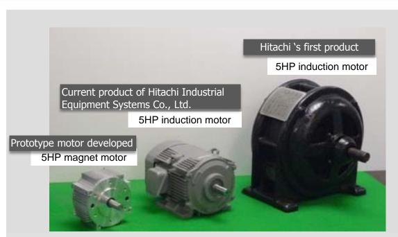
How small can we make Hitachi's original product, "the 5HP induction motor," using today's advanced technology?
